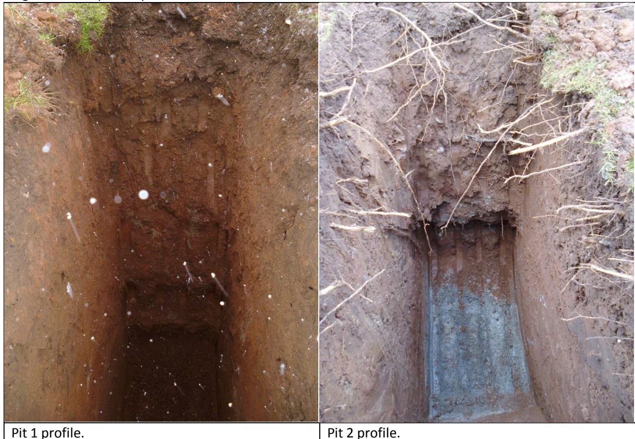
Figure 4. Trial pit soil profiles
