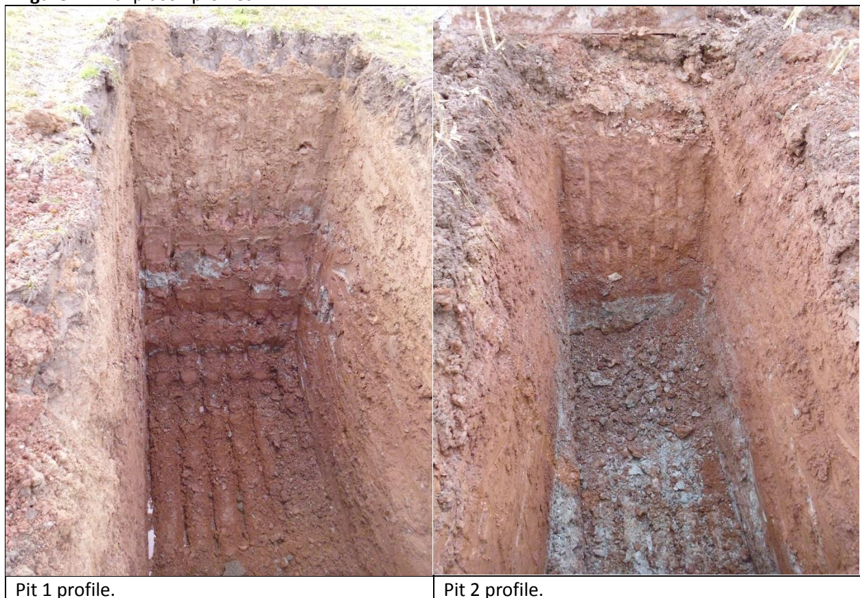
Figure 4. Trial pit soil profiles
