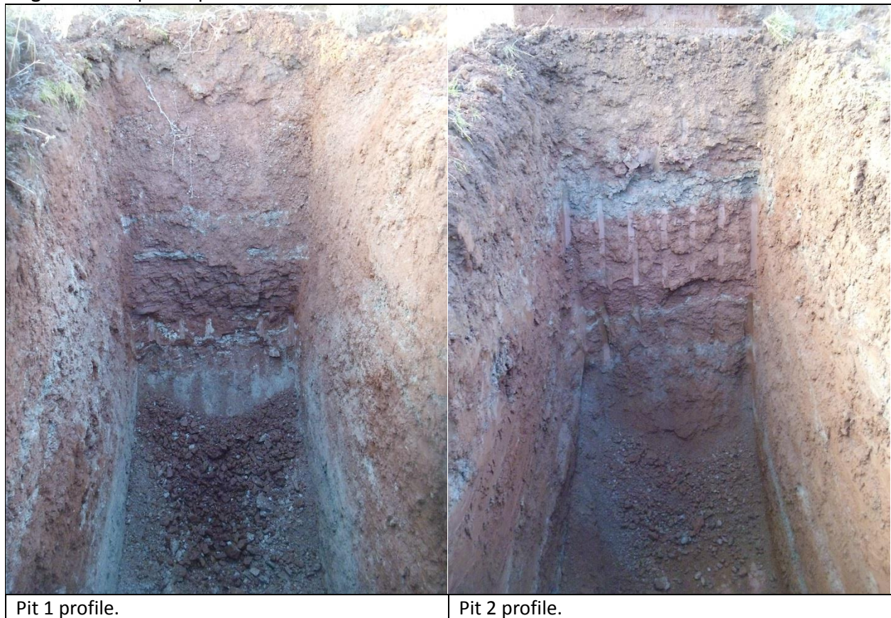
Figure 4. Trial pit soil profiles
